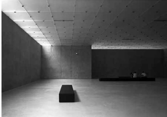
Initially we planned to direct daylight into the building through obliquely placed facade slats. Tested on models, this solution proved unsatisfactory. The best results were obtained by using etched glass shingles that refract the light before it enters the building. No matter what direction the light is coming from, it is always transmitted horizontally into the interior. Therefore, we placed a cavity above every floor to catch the light coming in from all four sides.
